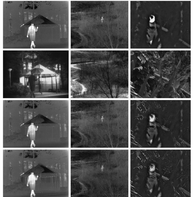
Fig. 7. From left to right: Kaptein_1654 , sand path and bush . From top to bottom: infrared image, visible image, fusion results of model without detail loss, and fusion results of model with detail loss.
