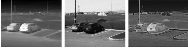
Fig. 15. Schematic illustration of low SSIM. From left to right: infrared image, visible image, and our fusion result.
