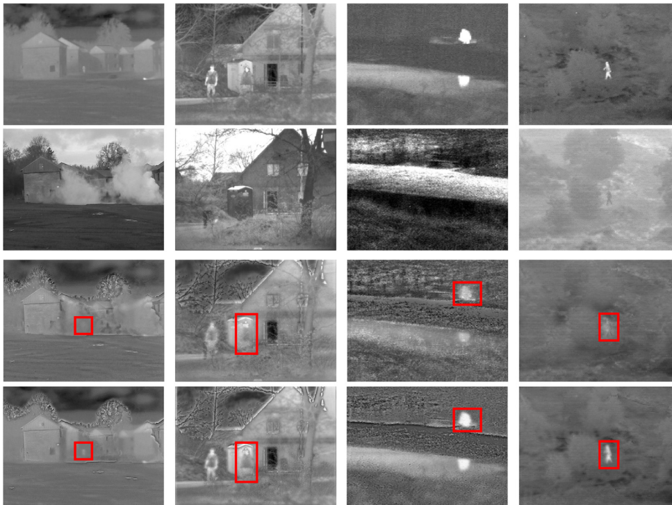
Fig. 4. Comparison of using pre-trained VGG-Net and discriminator as feature extractor on some typical infrared and visible image pairs. From left to right: smoke , men , bench and tree . From top to bottom: infrared image, visible image, fusion results of using VGG-Net as feature extractor, and fusion results of using Discriminator as feature extractor.
