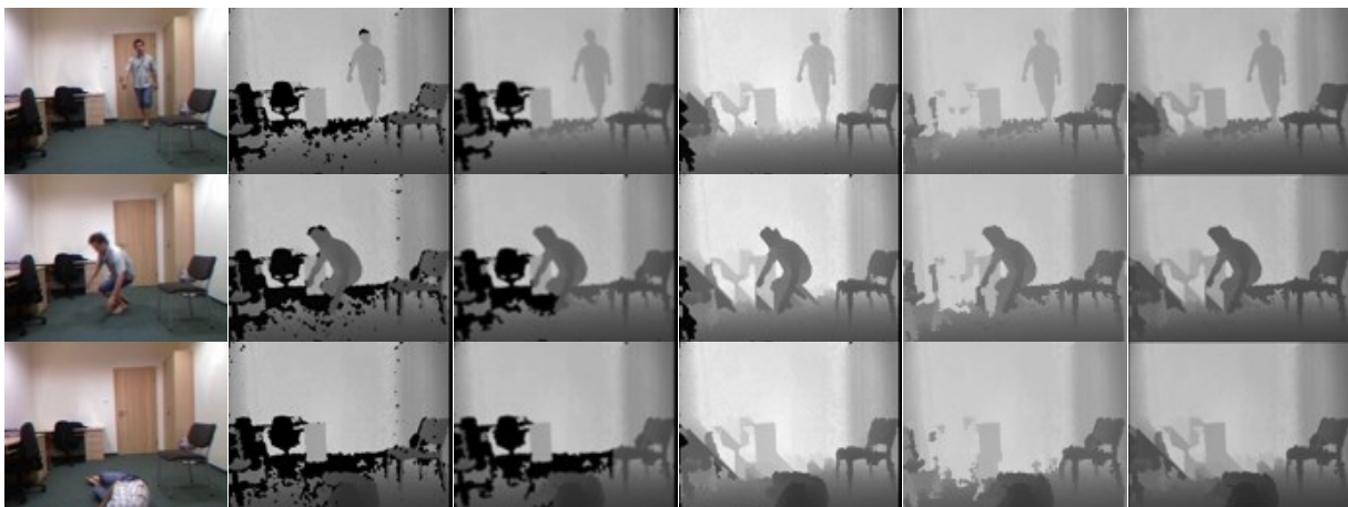
Fig.9 - Three sample frames of sequence 1: each row from left to right corresponds to the original color image, original depth map, recovered depth maps using JBF, FMM, GFMM, and the developed method
