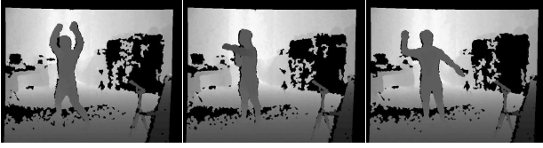
Fig. 1. Example depth images of the actions (left to right) jumping jacks , punching , and throwing a ball .
