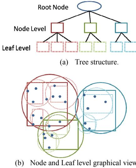
Fig. 2: Tree structure defined by the intersection of bounding spheres and bounding rectangles.
