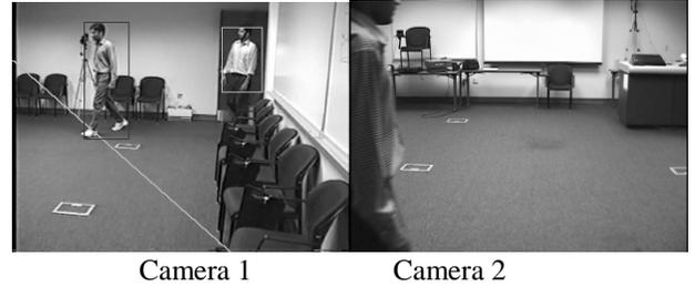
**Figure 1:** Example of correct handoff: There are two persons visible in Camera 1. When one of them enters the FOV of Camera 2, the left edge of FOV of Camera 2 as seen in Camera 1 ( $L^{21}_l$ ) helps us disambiguate between the labels.
