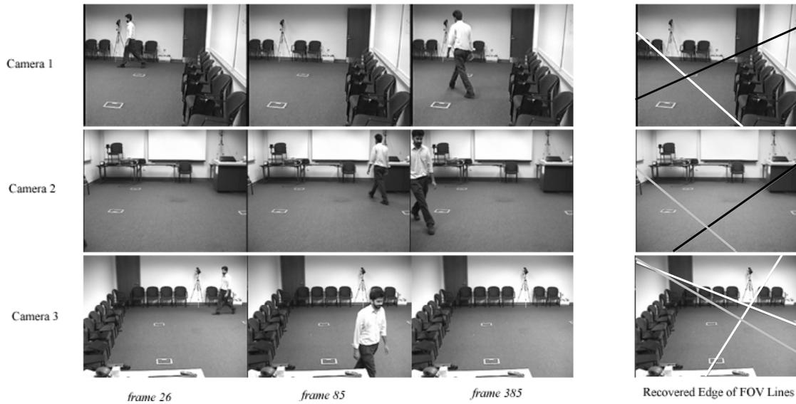
**Figure 5:** Determination of Edge of FOV lines using a short sequence of person walking in the room. The first 3 columns show triplets of sample images taken at same time instant. The last column shows the recovered lines
