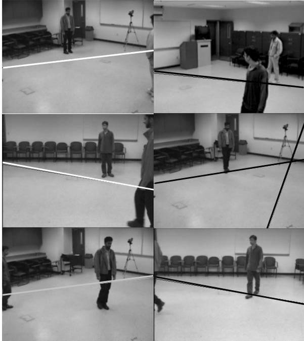
**Figure 7:** Handoff examples in Sequence 2. In each of the cases in column 1, a person is entering a new camera. By looking at images in the 2<sup>nd</sup> column, we can correctly identify this person.
