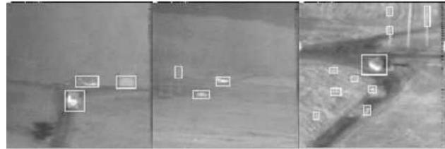
Fig. 2. Target candidates detected using the fuzzy clustering and edge fusion.
