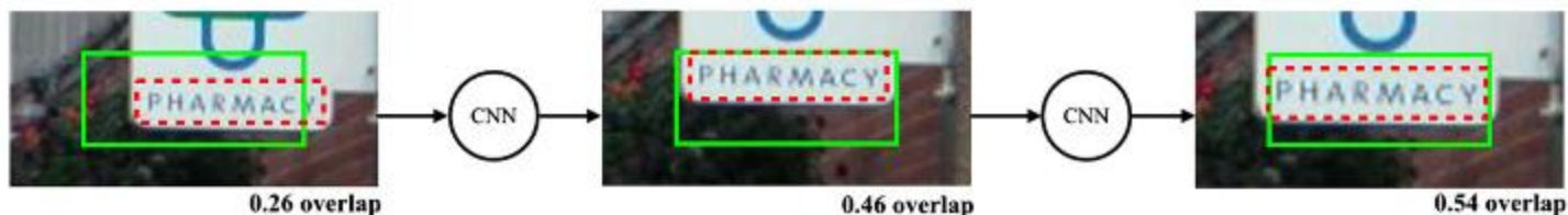
An example of the improvement in localisation of the word detection pharmacy through multiple rounds of recurrent regression
